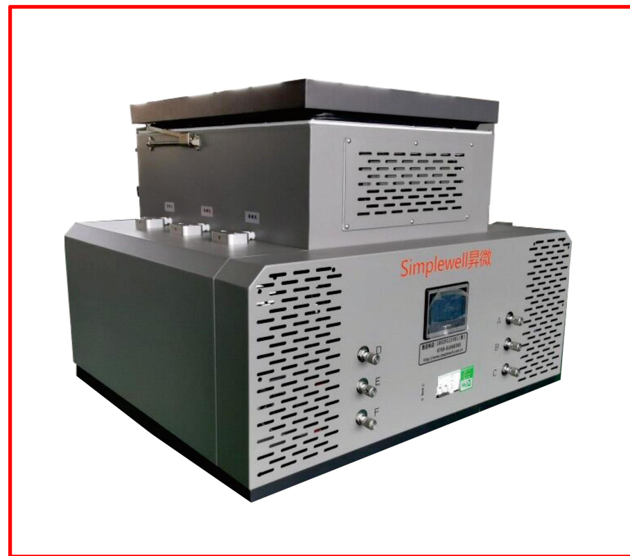
SVOC micro emission chamber
