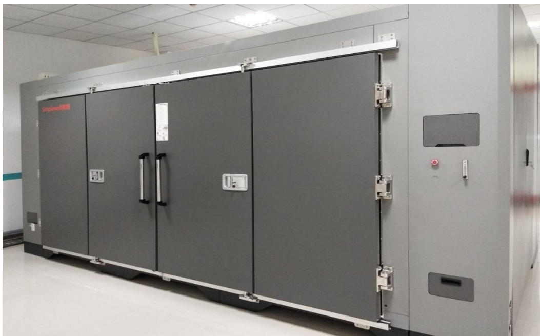
Evaporative pollutant environmental chamber
