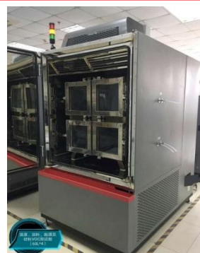
VOC emission chamber for outdoor product
