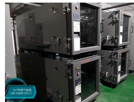
1m³ formaldehyde emission chamber
