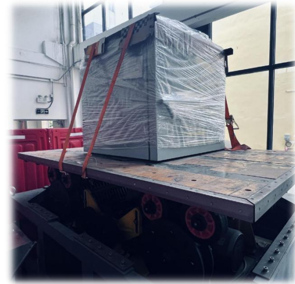
Vibration test for small equipment before shipment
