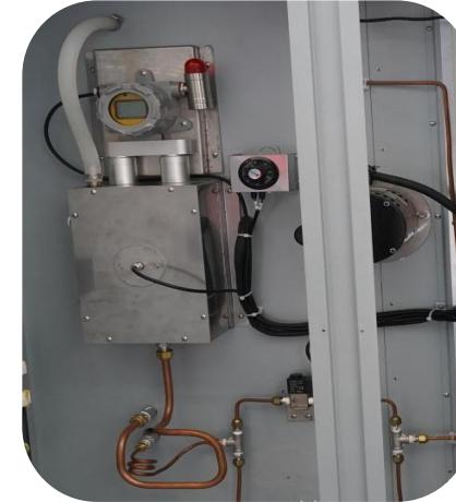
Fire extinguishing device and explosion-proof device (Battery high temperature chamber)
