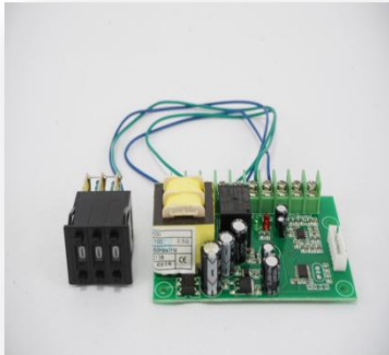
Independent over-temperature protection Control of upper temperature limit
