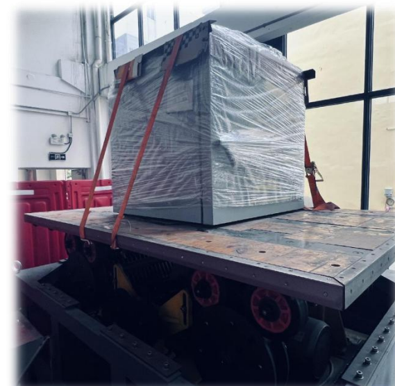
Vibration test for small equipment before shipment
