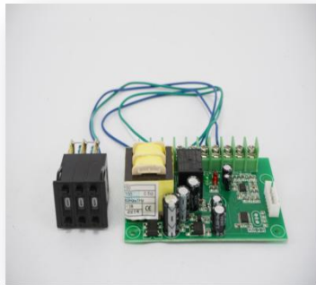
Overtemperature protection (Yatai)
