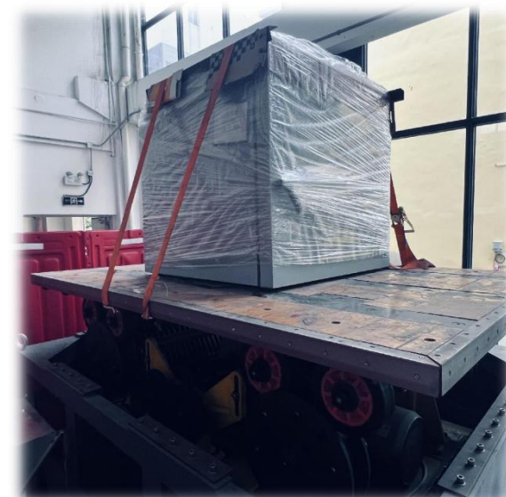
Vibration test for small equipment before shipment
