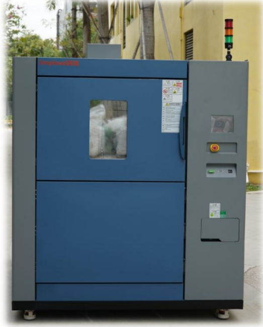
Two zone thermal shock chamber
