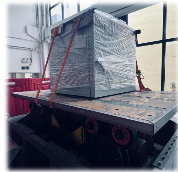
Vibration testing of small equipment prior to shipment
