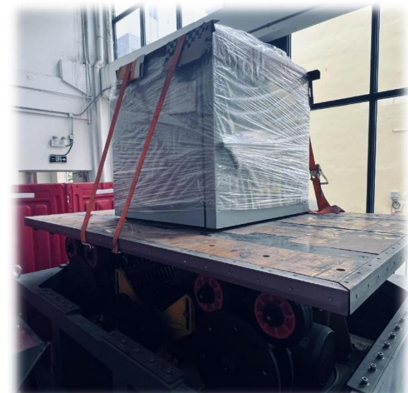
7. Vibration testing of small equipment prior to shipment
