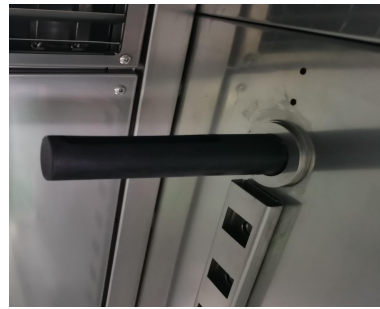
Plastic Humidity Sensor (LSTH/LNTH)
