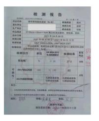
Flame-retardant warehouse boards and materials are used. The picture shows the performance test report of the warehouse board's flame retardancy, compressive strength, bending load-bearing capacity, etc.
