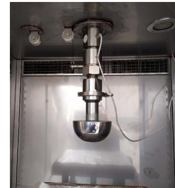
Servo electric cylinder propulsion The seamless inner cylinder bears high pressure, safe and reliable
